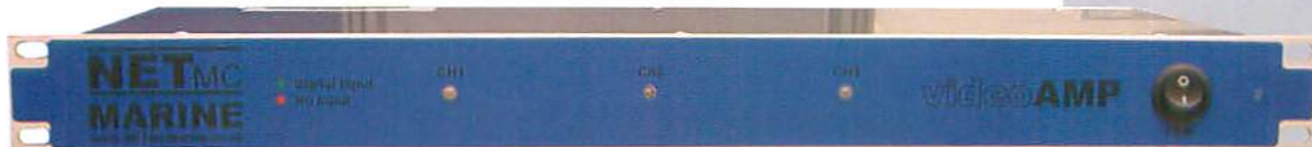
Front panel bi-colour LEDs show channels with valid input signals.
